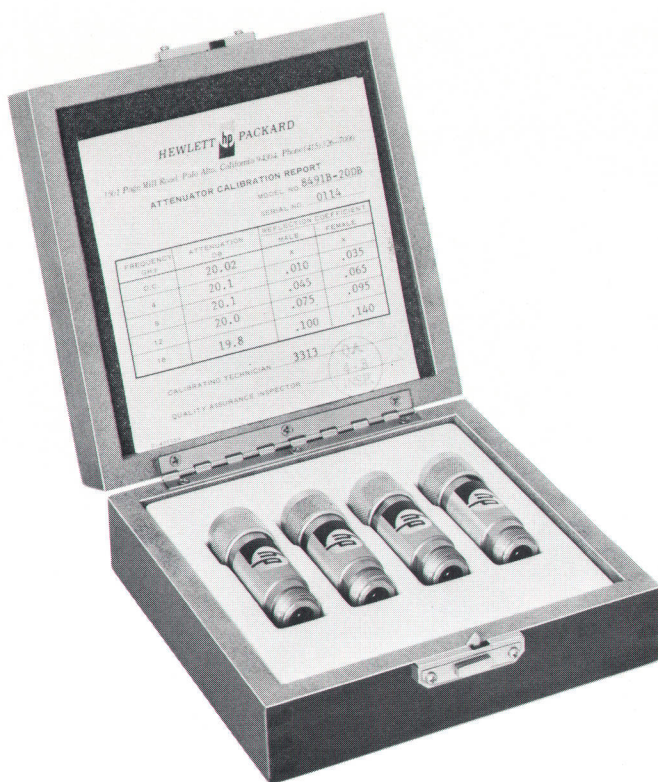
Fig. 9. Fixed attenuators were designed to be used singly or in sets of four — one each of 3, 6, 10, and 20 dB values. Sets contain calibration reports for all four attenuators.
