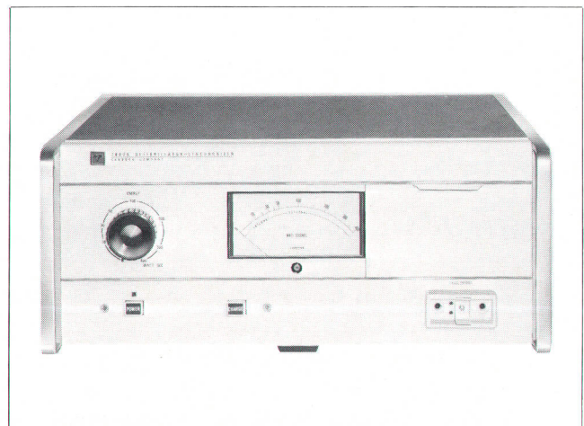
Fig. 9. Defibrillator produces up to 400 joules in a dc pulse typically applied to heart through chest wall.
