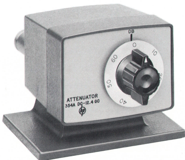
Fig. 10. HP Model 354A 0-to-60 dB Coaxial Step Attenuator uses thin-film attenuating cards. Frequency range is dc to 12.4 GHz.
