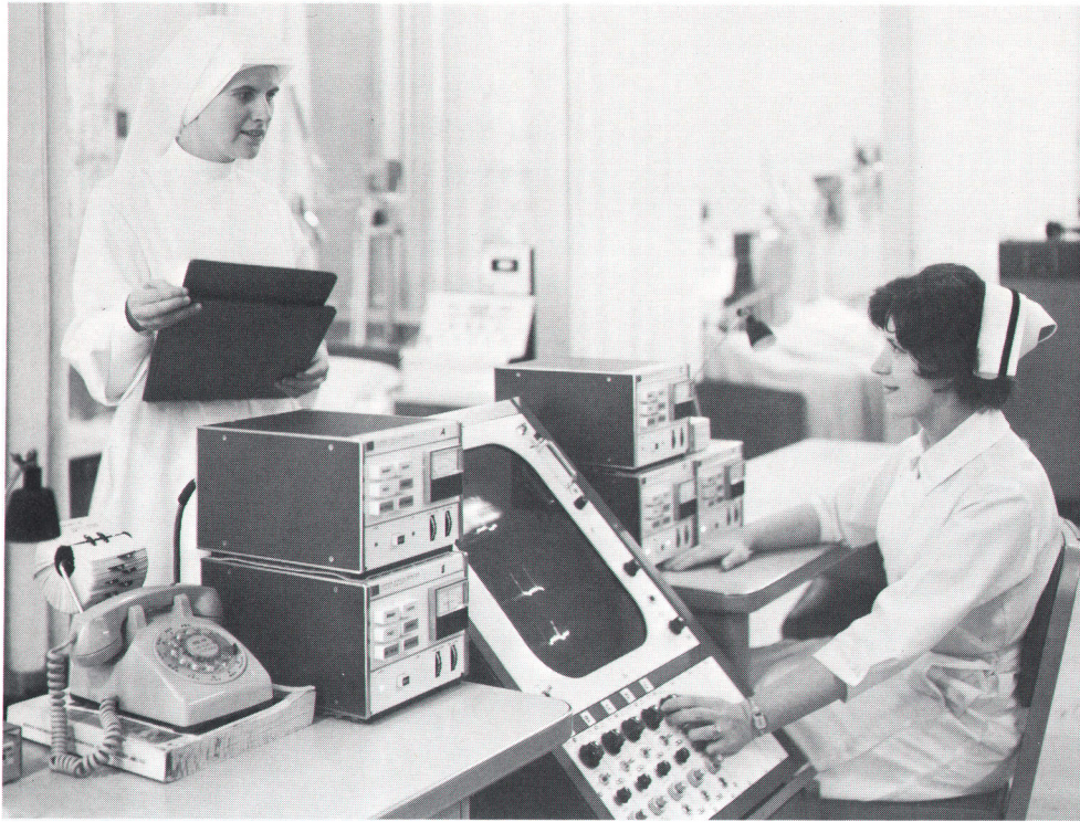
Fig. 2. Typical central station patient-monitoring equipment. Heart-waveforms are displayed on large-screen Sanborn scope. Alarm equipment is also provided to signal low or high heart rates, etc. Patient rooms are often arranged so that nurse always has patients in view.
